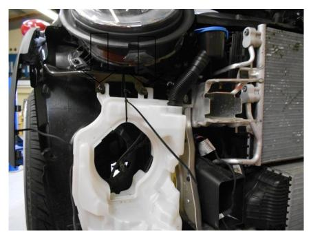
18. Using a flat blade screwdriver or similar remove the 2x clips inside the wheel arch. Using T27 Torx driver undo the 1x screws. Lift the duct upwards to release it and remove it from the vehicle.
