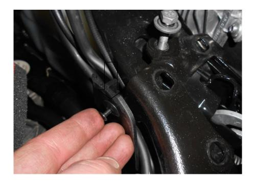
22. Undo the 2x radiator pins using a screwdriver or T30 Torxs driver.
