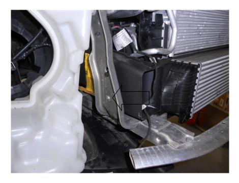
19. Undo the 5x T30 Torx bolts around each bonnet catch; do not fully remove the bolts.
