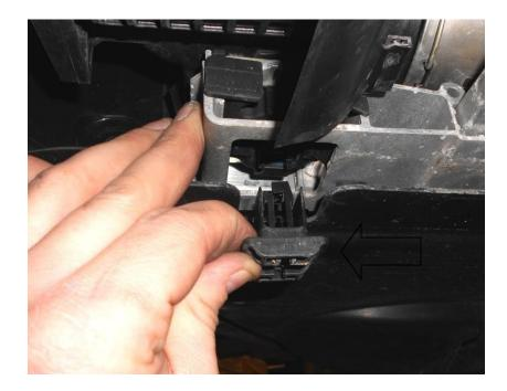
26. This next part requires 2 people. Lift the intercooler and radiator pack upward to release the intercooler from the bottom rubber mounts. Use a flatblade screwdriver or similar tool to release the rubber mounts if necessary.
