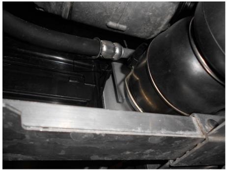
31. Using the 2x M6X16mm Allen cap bolts and 2x 6mm washers align and secure the radiator to both intercooler brackets.
