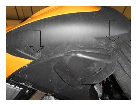
4. Using 8mm socket and suitable ratchet undo the 1 off screw inside each wheel arch. Rotate the access panel inside the wheel arch and unclip wiring to the back of the fog light on both sides.
