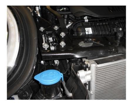
20. Using a 10mm socket and suitable ratchet remove 1x bolt.
