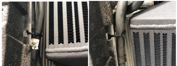
34. Follow steps 1 to 22 in reverse to reassemble your vehicle. The active air ducting (if fitted) in step 10, is not refitted as part of this installation. Use a cable tie or similar secure any loose wires.
