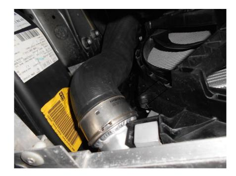
33. If fitting to the 2019- GP3 the extra auxiliary hoses need to be cable tied to the crash bar to avoid rubbing as pictured below.
