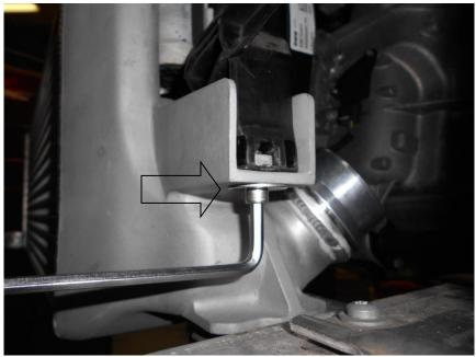
32. Re-connect both intercooler hoses. Ensure that the spring clips are fully released and have fully engaged in the recess in the CNC coupler. If these are not correctly installed they may come off during normal driving.
