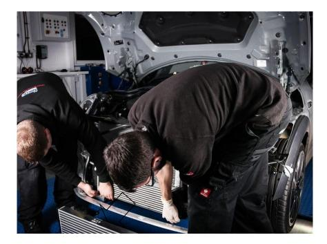
28. Fit the radaitor mounts into the brackets on both end tanks of your Forge intercooler before lifting the intercooler upwards and pushing the bottom edge backward to allow the mounting pegs to locating the rubber bushes.
