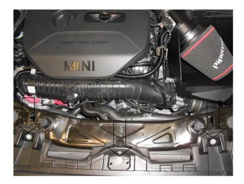
9. Unclip the sensors at each end of the crash bar and remove the foam crash bar cover. Note: <u>DO NOT SWITCH ON</u> THE IGNITION WITH THIS DISCONNECTED AS IT WILL CAUSE A WARNING LIGHT ON THE DASH WHICH CAN ONLY BE RESET AT A BMW DEALER.
