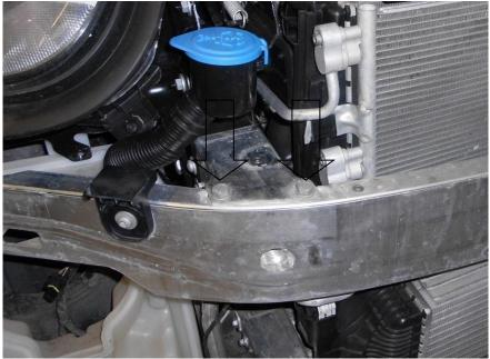
15. From inside the wheel arch using a flat blade screwdriver or similar tool remove the 2x clips. Pull the centre out first before removing the body of the clip.
