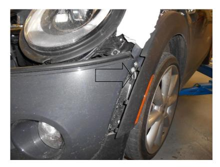
7. If your vehicle is fitted with Spot lights use a 3mm Allen key to loosen the horizontal bolt. Tilt the light forward using a 2mm Allen key undo the bolt and remove the headlight. Note the next part requires 2 people as the wiring connectors can only be undone once the bumper has been removed from the vehicle.
